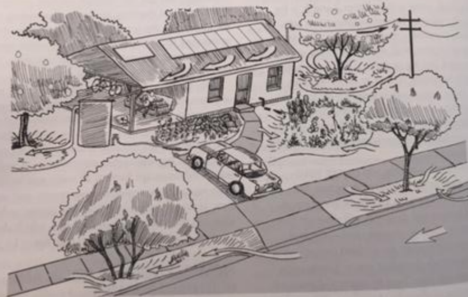
Fig. 1.1B. A home and landscape harvesting and producing resources. White arrows denote runoff flow. Black arrow denotes electricity flow. Dotted lines denote greywater pipe. Solar panels and solar hot water heater added to roof
